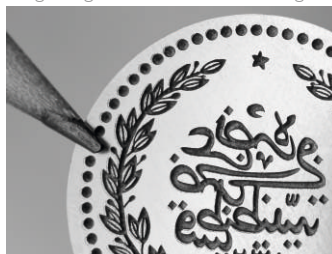
Engraving on Harden cold working SS
