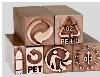
Deep Engraving on Copper Electrode
