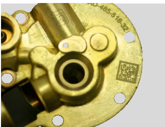
Step Marking on Brass
