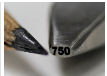
Micro Engraving on Hardened SS
