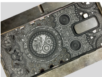
3D Engraving on Mobile Die
