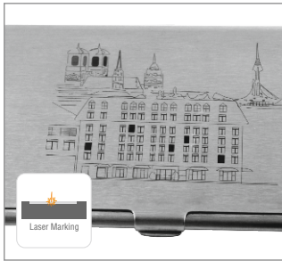
Laser Marking on Metal
