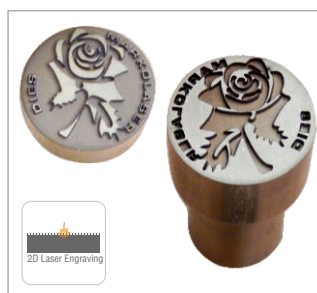
Deep Engraving of Male-Female Embossing Punch Dies
